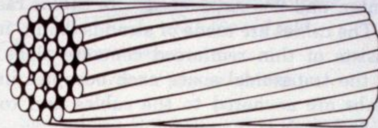
(a) Galvanized Bridge Strand
